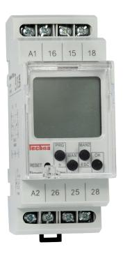
The Timetec-RTAstro is a 2-channel Time Switch used for controlling different loads according to sunrise and sunset times based on geographical location. The Time Switch can be used to control various appliances in real time, such as, switching of heating, pumps, ventilation systems etc. The timer operates all year round without the need for maintenance, with minimum operating costs and maximum savings of electrical energy.
